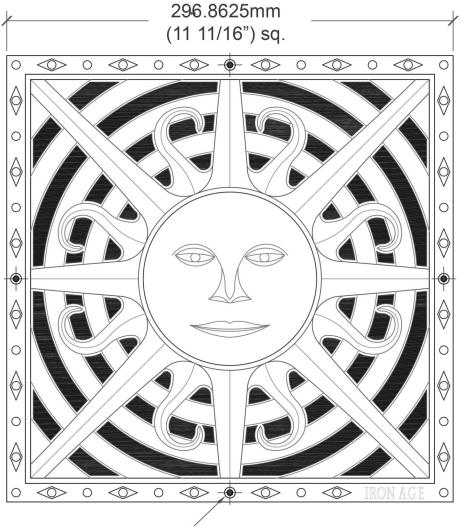
(x4) Divots to locate bolt - down holes as desired
